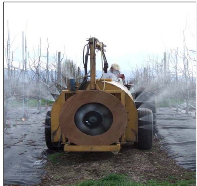
Airblast sprayer fitted with two-thirds area plywood donut
