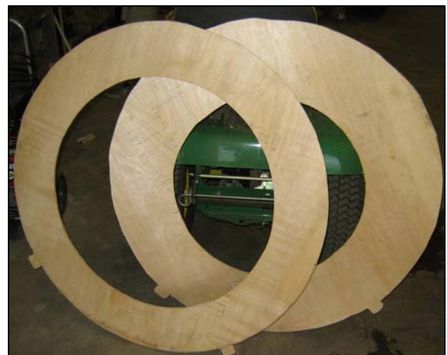
Plywood donuts of one-half (front) and two-thirds (rear) the area of fan intake.
